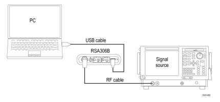
Figure 2: Instrument connections
