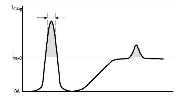
**NOTE.** Always degauss the probe after measuring a current that exceeds the maximum continuous current, maximum pulsed current, or Ampere-second product rating of the probe. Exceeding these ratings can magnetize the probe and cause measurement errors.
