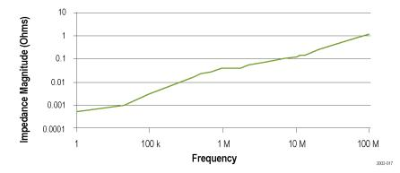
Figure 2: Typical input impedance versus frequency
