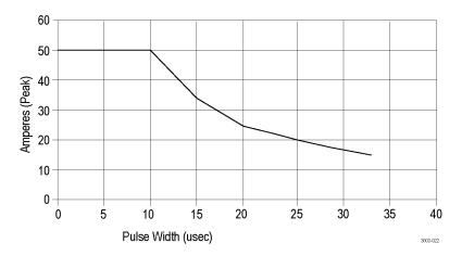
Figure 3: Maximum peak pulse versus pulse width
