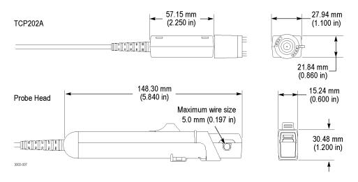
Figure 4: Probe dimensions
