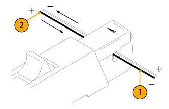
**NOTE.** Adding a second conductor to the probe increases the insertion impedance and reduces the upper bandwidth limit of the probe. Winding multiple turns further increases the insertion impedance, further reducing the upper bandwidth limit.
