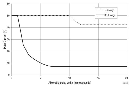
Figure 3: Maximum peak pulse versus pulse width
