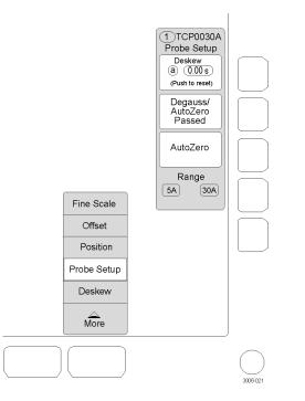
**Deskew.** To deskew the TCP0030A probe to other probes, select this function and connect the probes to the optional deskew fixture. (See page 43, *Deskew/Calibration Fixture.*)
