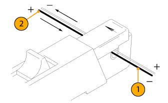
**NOTE.** Adding a second conductor to the probe increases the insertion impedance and reduces the upper bandwidth limit of the probe. Winding multiple turns further increases the insertion impedance, further reducing the upper bandwidth limit.
