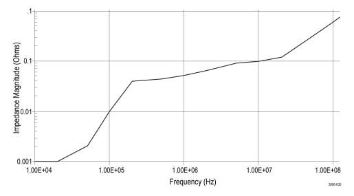
Figure 2: Typical input impedance versus frequency
