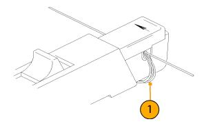
NOTE. Winding more turns around the probe increases the insertion impedance and reduces the upper bandwidth limit of the probe.
