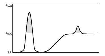
Ampere-Second Product is the maximum width of pulsed current that you can measure when the pulse amplitude is between the maximum continuous and maximum pulsed current specifications. The maximum continuous specification varies by frequency.
