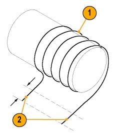
NOTE. Ensure that the current loop has exactly 5 turns. A significant error will result for each turn variance from 5 turns.
