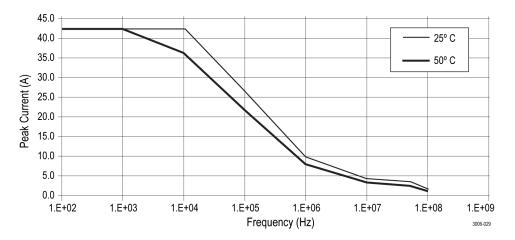
Figure 1: Frequency derating (peak current versus frequency)
