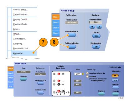
10. Oscilloscopes that support the automated TriMode calibration routine will display an on-screen prompt to toggle the Calibration Fixture SIG/GND switch. Follow the instructions to complete the calibration for the remaining input modes.
