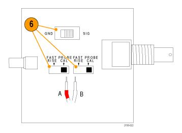
Table 3: TriMode DC Calibration board switch settings
