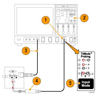
**6.** Set the switches on the TriMode DC Calibration board to the positions shown for the selected input mode. (See Table 3.)
