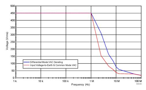
Figure 7: P5202A voltage derating curve
