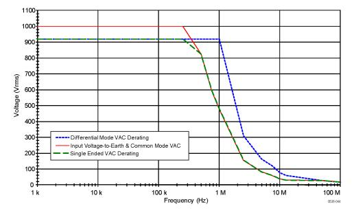
Figure 6: P5200A and P5205A voltage derating curves
