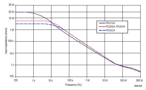
Figure 5: P5200A Series impedance plots
