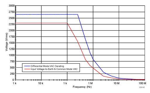
Figure 8: P5210A voltage derating curve
