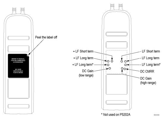
Figure 14: Internal adjustment locations (S/N C020000 and above only)
