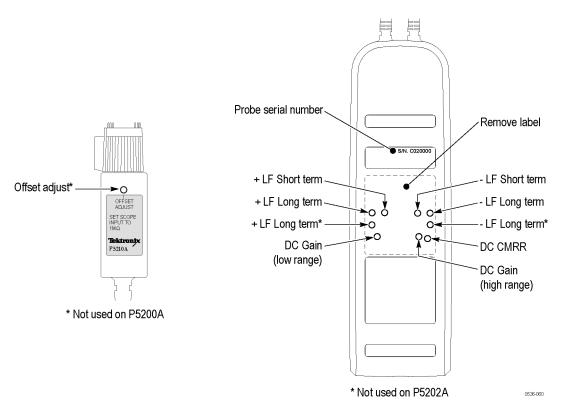
Figure 13: P5200A Series probe serial number and adjustment locations
