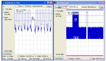
Swept DPX combines the revolutionary DPX Density<sup>™</sup> Trigger with the ability to trigger on runt pulses and apply time qualification to any trigger. The runt trigger seen here can be used to track down nonconforming pulses in a pulse train, greatly reducing time to insight. Time qualification can be used to separate ranging pulses from higher resolution pulses in a radar signal, or trigger only on signals that remain on longer than a specified time.
