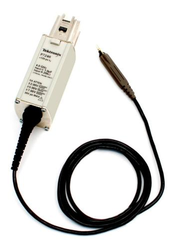
The P7240 4 GHz, 5X active FET probe provides truer signal reproduction and fidelity for high-frequency measurements. The probe has low input capacitance and high input resistance to minimize circuit loading over a wide bandwidth range.
