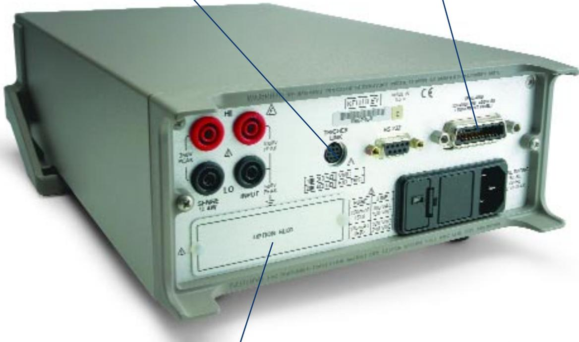
Built-in scanner mainframe accepts optional switching cards for multi-point testing
